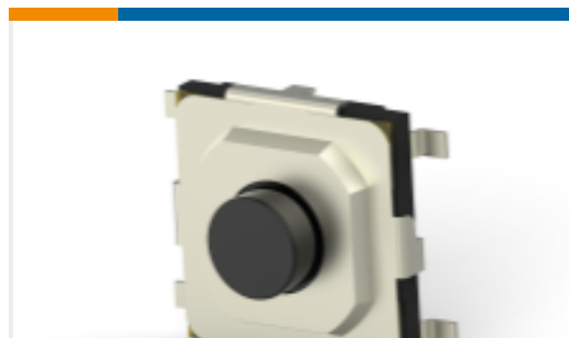
TE Part #2337238-3 TACT MINI GW 5.2X5.2X2 160GF
