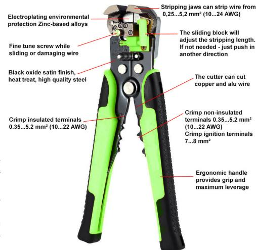
This automatic multifunction wire stripper is particularly suitable for hobbyists, craftsmen, field service, service workshops, electronics technicians and laboratory needs. The tool provides a lot of helpful functions and is made of high quality materials.
