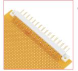
connect to 31-pin plug connector (DIN 41617)
