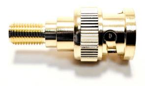
• The BU-P4289 is a BNC male to SMA female adapter typically used in RF applications. The SMA end of the adapter uses a 1/4-36 UNS-2A thread.
