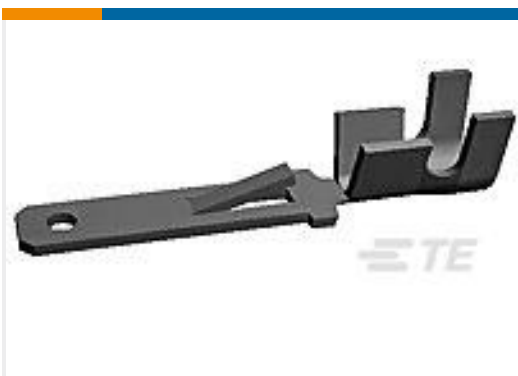
TE Part #170014-5 FF 110 TAB 20-16AWG BR
