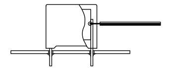
Temperature monitored inside the capacitor.
