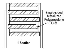
Film Capacitors - Polypropylene Pulse/High Frequency Capacitors
