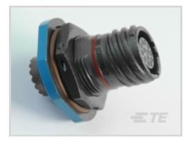
Connector System: Cable-to-Panel Number of Positions: 19 Sealable: Yes Connector & Contact Terminates To: Wire & Cable Contact Current Rating (Max): 23 A
