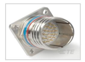
Connector System: Cable-to-Panel Number of Positions: 32 Sealable: Yes Connector & Contact Terminates To: Wire & Cable Contact Current Rating (Max): 7.5 A
