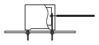
Temperature monitored inside the capacitor.
