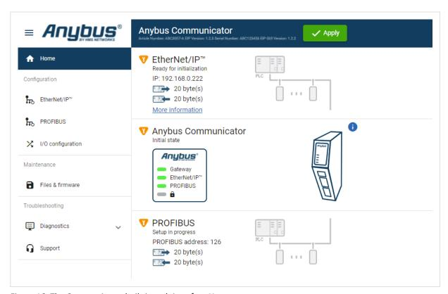
Figure 16. The Communicator built-in web interface Home page
