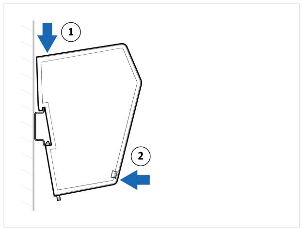
Figure 4. Attach the Communicator on the DIN rail
