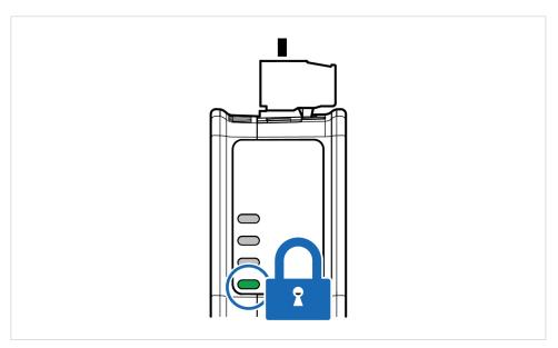
Figure 12. Security switch locked status LED
