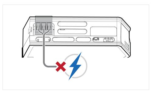
Figure 8. Disconnect Communicator from power
