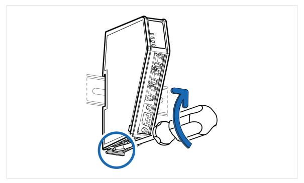
Figure 14. Unlock the Communicator
