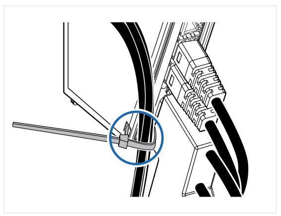
Figure 13. Lock the cables
