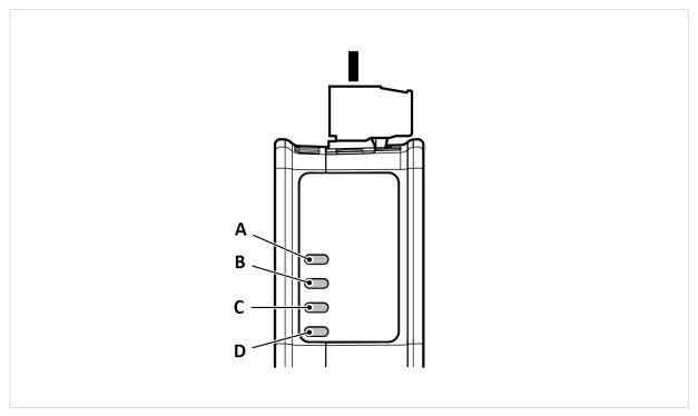
Figure 37. Gateway status (A), Lower connector (B), Upper connector (C) and (D) Security Switch
