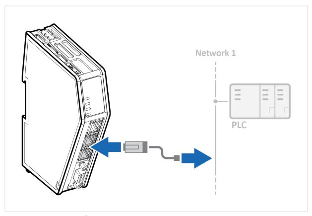
Figure 5. Connect to EtherNet/IP network
