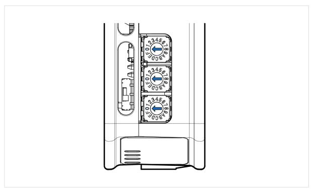
Figure 7. Rotary switches default setting **000**.
