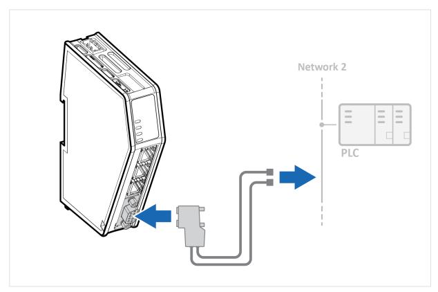
Figure 6. Connect to PROFIBUS network
