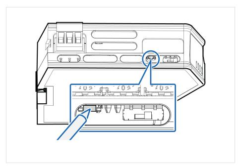
Figure 46. Press and hold **Reset** button
