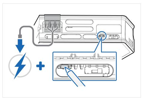
Figure 47. Hold Reset button and reconnect power
