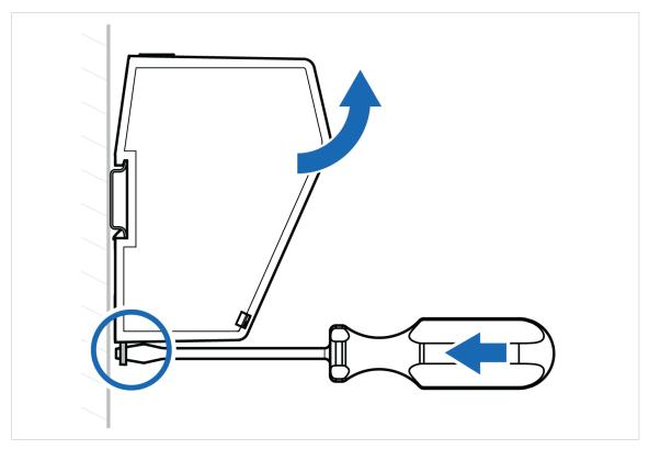
Figure 15. Unhook the Communicator
