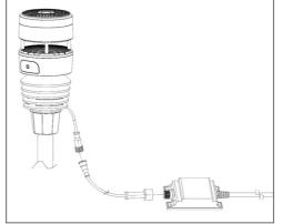
If expansion plugs are needed to fix the power adapter at the chosen place of installation (depending on the surface texture), mark the exact position of the four drill holes through the mounting holes of the power adapter.
