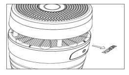
First, loosen the fixing nut on the underside of the outdoor sensor (N).
