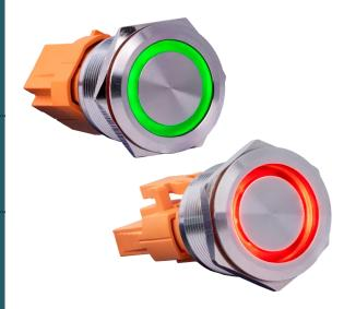
Our momentary / latching steel push button convinces with high-quality materials, protection classes and ergonomics. It is made of stainless steel and meets the protection classes IP67 (dust and water), IK10 (impact) and PA66 (flame). The protection classes, the wide temperature range and the durability make our steel push button suitable for many applications. The steel push button has a bright LED ring (red / green).
