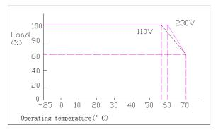
Input voltage Load derating curve
