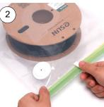
2.Try to remove some air and then seal the vacuum bag using a sealing clip.
