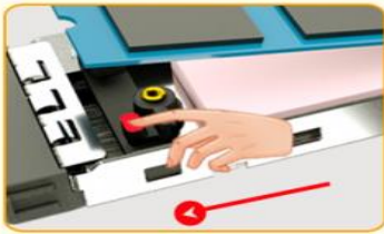
Push the front angle hook and press downward the M.2 SSD
