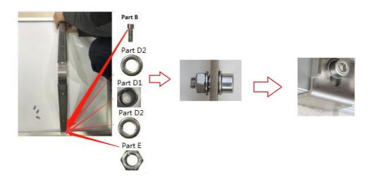
Refer to the above step, install the other 1PC Part C on the other side of the solar panel.
