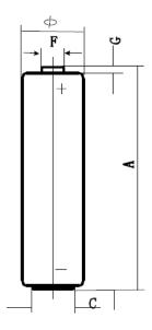
Capacity: 3000 mAh (10 mA, 24 h/d, 20°C, end voltage = 0.8 V)
