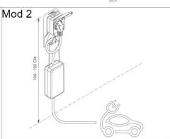
It is recommended to have the installation of a 3 x 2.5 mm<sup>2</sup> additionally fused cable carried out and checked by a qualified electrician.
