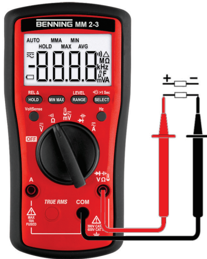
Figure 11: Resistance measurement or continuity test
