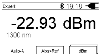
Fig. 3 Display in Auto-λ mode showing one detected wavelength and the power level.
