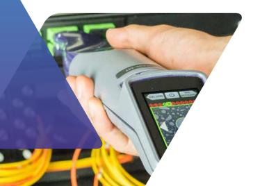
FiberChek Sidewinder is the fastest and easiest MPO inspection solution there is. Simply insert it into the bulkhead, press a button, and the Sidewinder will provide automatic results for all 12 MPO fibers in fewer than 12 seconds!
