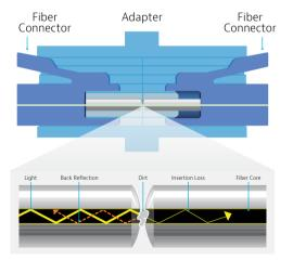
Inspecting BOTH sides of the fiber connection is the only way to ensure that it will be free of contamination and defects, and prevents cross-contamination.. VIAVI fiber optic probe microscopes allow inspection of both male and female optical connectors.
