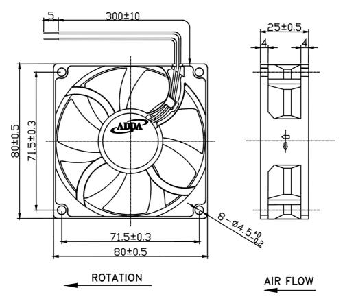
LEAD WIRES: UL 1007, AWG24, L = 300±10 mm Red = positive; Black = negative.
