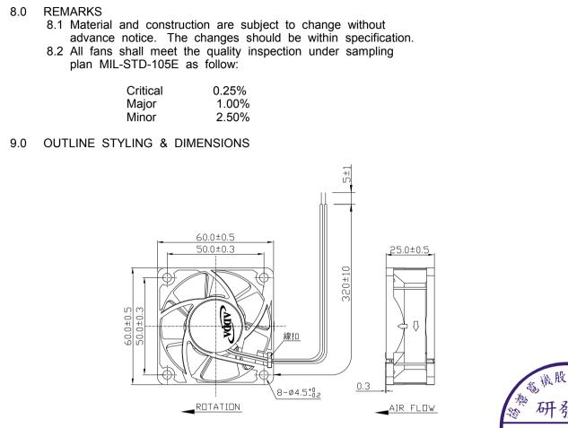
LEAD WIRES : UL 1007, AWG24 , L = 320 +/- 10 mm Red = positive ; Black = negative.
