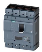
circuit breaker 3VA2 IEC frame 630 breaking capacity class L Icu=150kA @ 415V 4-pole, line protection ETU850, LSI, In=630A overload protection Ir=250A...630A short-circuit protection Isd=0.6..9x In, Ii=1.5..9x In N conductor protection adjustable (OFF, up to 100%) nut keeper kit
