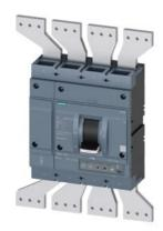
circuit breaker 3VA2 IEC frame 1250 breaking capacity class C lcu=110kA @ 415 V 4-pole, line protection ETU350, LSI, In=1250A overload protection Ir=500A ...1250A short circuit protection Isd=1,5... 10 xIr, li=10 x In N conductor protection adjustable (OFF, up to 100%) nut keeper kit
