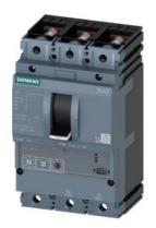
circuit breaker 3VA2 IEC frame 160 breaking capacity class E Icu=200 kA @ 415 V 3-pole motor protection ETU350M, LSI, In=25A overload protection Ir=10A ... 25A short circuit protection Isd=3...15xIr, Ii=15xIn busbar connection
