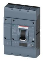
circuit breaker 3VA6 UL frame 1000 breaking capacity class H 65kA @ 480 V 4-pole, line protection ETU556, LSI, In=1000A overload protection Ir=400A ...1000A short circuit protection Isd=0,6...10x In, Ii=1,5...10x In
