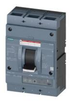
Circuit breaker 3VA6 UL Frame 800 breaking capacity class H 65kA @ 480 V 3-pole, Line protection ETU320, LI, In=800A overload protection, 100% rated Ir=315A ...800A Short-circuit protection Ii=1.5...10 x In Nut keeper kit
