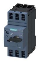
circuit breaker size S00 for transformer protection without phase failure protection A-release 3.5...5 A short-circuit release 104 A spring-loaded terminal standard switching capacity
