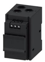
Current/voltage measuring module for dry-running protection of centrifugal pumps in hazardous areas; set current 10 ... 115 A, voltage measurement up to 690 V, width 55 mm, straight-through transformer
