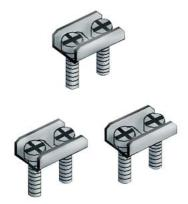
accessory for In-line fuse switch disconnectors 3NJ4103 Kit saddle terminal CU 1.5 to 70 mm2 1 set = 3 units
