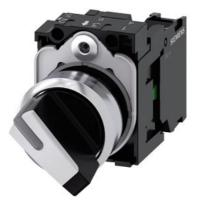
Toggle switch, 22 mm, round, metal, shiny, white, knob, short, 2 switch positions O<I, momentary contact type, actuating angle 45°, 10:30h/12h, with holder, 1 NO, screw terminal
