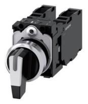
Toggle switch, 22 mm, round, metal, shiny, white, knob, long, 3 switch positions I>O<II, momentary contact type, actuating angle  $2x45^\circ$ , 10:30h/12h/13:30h, with holder, 1 NO, 1 NO, screw terminal
