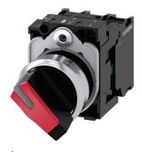
Toggle switch, illuminated, 22 mm, round, metal, shiny, red, knob, short, 2 switch positions O-I, latching, actuating angle 90°, 10:30h/13:30h, with holder, 1 NO, 1 NC, LED red, 24 V AC/DC, screw terminal
