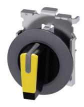
Selector switch, illuminable, 30 mm, round, metal, matte, yellow, selector switch, short, front ring for flush installation, 3 switch positions I-O-II, latching, actuating angle  $2x45^{\circ}$ , 10:30h/12h/13:30h
