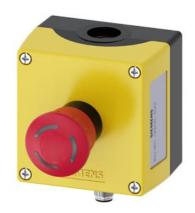
Enclosure for command devices, 22 mm, round, enclosure material plastic, enclosure top part yellow, 1 control point plastic, A=EMERGENCY STOP mushroom pushbutton red, 40 mm, rotate-to-unlatch, illuminated, 2x 1 NC, LED white 24 V, spring-type terminal, floor mounting, M12 connector (8-pole) bottom, insulated reserve conductors Pin assignment: PIN1=11, PIN2=12, PIN3=21, PIN4=22, Pin5=n.c., Pin6=n.c., Pin7=ground LED, PIN8=LED, one connection at 1 input F-DI, one connection at 1 output F-DQ
