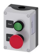
enclosure for command devices, 22 mm, round, enclosure material plastic, enclosure top part gray, 2 control points plastic, B=Pushbutton green, label: start, 1 NO, screw terminal, A=Mushroom pushbutton red, momentary contact type, label: Stop, 1 NC, screw terminal, floor mounting, 1xM20 each on top and bottom, Labels glued in
