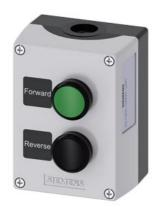
enclosure for command devices, 22 mm, round, enclosure material plastic, enclosure top part gray, 2 control points plastic, B=Pushbutton green, label: Forward, 1 NO, screw terminal, A=Pushbutton black, label: Reverse, 1 NO, screw terminal, floor mounting, 1xM20 each on top and bottom, Labels glued in
