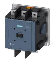
power contactor AC-1 900 A / 690 V / 40  $^{\circ}$ C 3-pole, Uc: 110-127 V AC(50-60 Hz) / DC drive: conventional auxiliary contacts 2 NO + 2 NC main circuit: busbar control and auxiliary circuit: screw terminal
