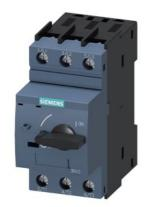
circuit breaker size S0 for starter combination rated current 16 A short-circuit release 208 A screw terminal standard switching capacity 30 kA at 600 V according to UL/CSA
