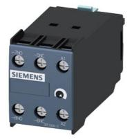
solid-state time-delayed front-side auxiliary switch Time range 5...100 s, 200 ... 240 V AC, 1 NO contact, 1 NC contact ON delay, for 3RT1
