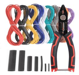
**Technical data (LIY Cu Wire):** Material: PVC insulation, copper wire • Rated voltage: 230 V AC/DC • Operating temperature range: -30 ... +70 °C • Lead-free • Halogen-free • RoHS-compliant • Colors in Set: white, blue, brown, orange, green, yellow, gray, purple, black, red. Details see list down below.
