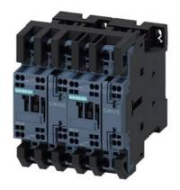
reversing contactor assembly, AC-3e/AC-3, 17 A, 7.5 kW / 400 V, 3-pole, 24 V DC, with integrated diode, spring-loaded terminal, electrical and mechanical interlock, auxiliary contacts: 2 x 1 NO
