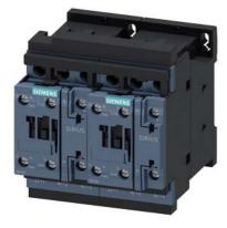
reversing contactor assembly, AC-3e/AC-3, 25 A, 11 kW / 400 V, 3-pole, 220 V AC, 50 Hz / 240 V, 60 Hz, screw terminal, electrical and mechanical interlock, auxiliary contacts: 2 x 1 NO
