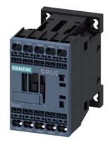
Coupling contactor relay railway 3 NO + 1 NC, 24 V DC, 0.7  $\dots$  1.25\* US, with varistor integrated, Size S00, Spring-type terminal upright mounting position
