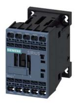
Coupling contactor relay, 4 NO, 30 V DC, 0.7  $\dots$  1.25\* US, with integrated diode, Size S00, Spring-type terminal suitable for PLC outputs
