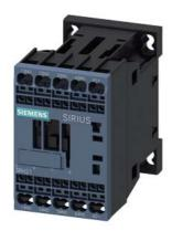
Coupling contactor relay railway 4 NO, DC 72 V, 0.7 ... 1.25\* US with integrated varistor, Size S00, Spring-type terminal
