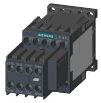
Contactor relay, 4 NO + 4 NC, 120 V AC, 50 / 60 Hz, Size S00, screw terminal, 2 NO + 2 NC basic unit / EN Varistor plugged on
