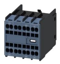
auxiliary switch, solid-state compatible, on the front, 2 NO + 1 NC, .3/.4, --/--, .3/.4, .1/.2, current path: 1 NO (solid-state compatible), --, 1 NO, 1 NC (solid-state compatible), spring-loaded terminal, for contactors 3RT2 and contactor relays 3RH2
