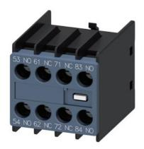
auxiliary switch, on the front, 2 NO + 2 NC, 53/54, 61/62, 71/72, 83/84, current path: 1 NO, 1 NC, 1 NO, screw terminal, for contactors 3RT2 and contactor relays 3RH2
